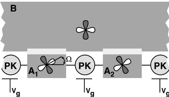
Fig. 1. Superconducting grain boundary qubits: Terminals  $A_1$ ,  $A_2$  and  $B$  are d-wave superconductors, PK (parity key) represent the SSETs,  $\Omega$  is the mismatch angle between the lattices of  $A_i$  and  $B$ . Positive lobes of the d-wave order parameter are shaded. Two physical qubits are shown.
