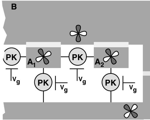
Fig. 11. Superconducting grain boundary qubits with “bus qubit”. The qubits are connected to the bus by SSETs.
