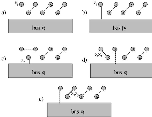
Fig. 10. (a) Implementation of logical  $X$  operation on logical qubit 1 is done by allowing physical qubit 1 to undergo free tunneling. This requires recoupling all other physical qubits in pairs as indicated by dashed lines. (b) Implementation of logical  $Z$  operation on logical qubit 1 is done by Josephson coupling physical qubit 1 to bus. This requires recoupling all other physical qubits in pairs as indicated by dashed lines. Similarly for (c),(d), and (e).
