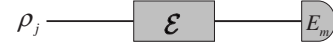
FIG. 1. Schematic of SQPT. An ensemble of states \{\rho_j\} are prepared and each of them is subjected to the map \mathcal{E} , and then to the measurements \{E_m\} .
