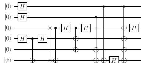
FIG. 1. Encoding circuit for the first six-qubit code. The  $H$  gate is a Hadamard gate. For example, we apply a Hadamard on qubit four followed by a CNOT with qubit four as the control qubit and qubit six as the target qubit.
